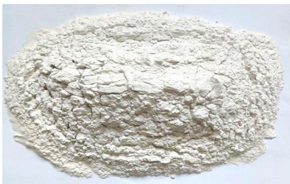
**Figure 7.** Potassium Permanganate and Starch Powders Mixture after 14 hour Blending
